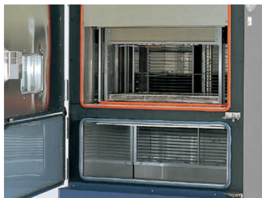
TSD-101-W Test areas ( Top: hot chamber Bottom: cold chamber )
